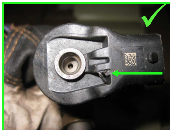
Carcasa electromagnet deteriorata → acceptabil
