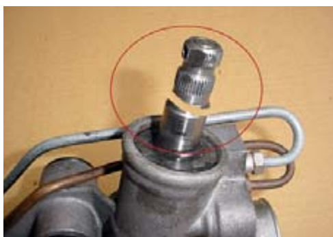
Arbore deteriorat sau rupt
